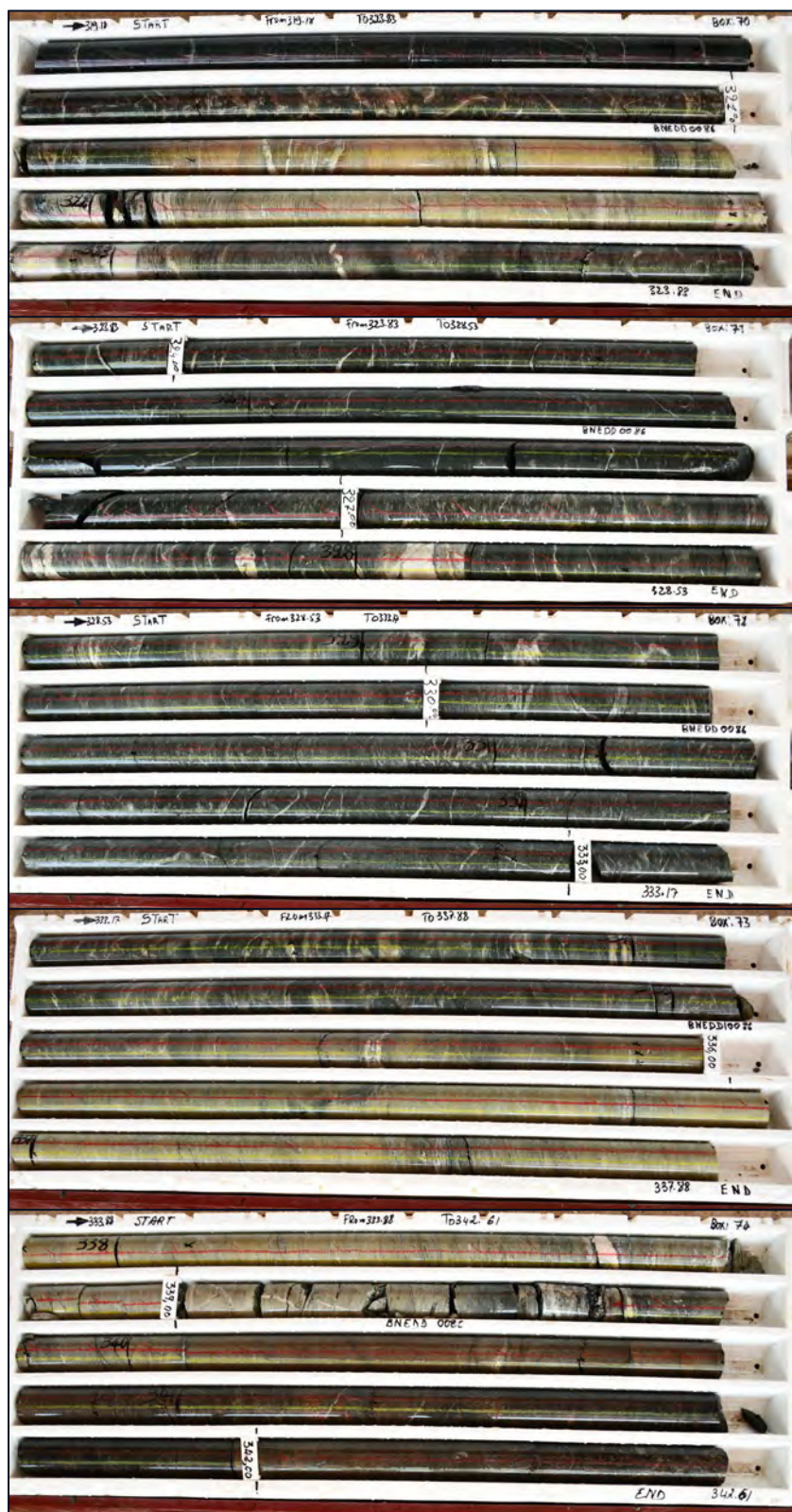
Figure 7.13: BNEDD0086 Main Shear 320.0-340.1m, 20.1m @ 0.48g/t
